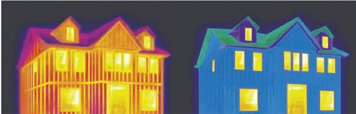
**Exterior Insulation is the most effective way to reduce thermal bridging with traditional stud framing.** Image: drivit.com
